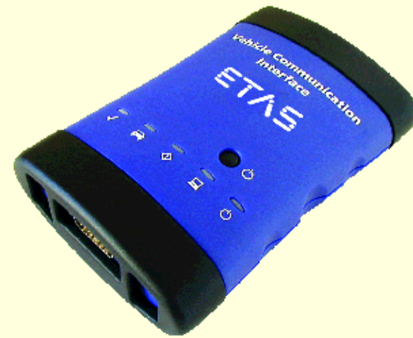
Figure 1: ETAS VCI (Vehicle Communication Interface) module for vehicle diagnostics.
